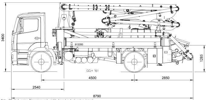
Note: Standard version. Dimensions and weights depend on truck and equipment. Dimensions in mm, MB-Axor 1828 as example.
