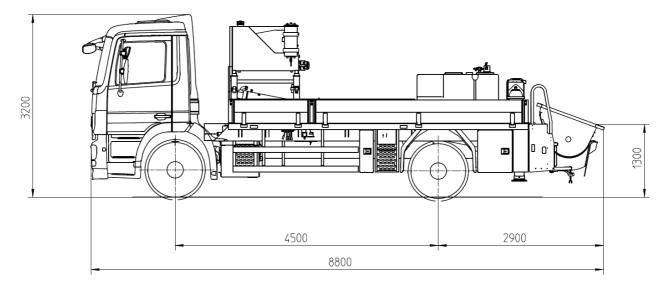
Note: Standard version. Dimensions and weights depend on truck and equipment. Dimensions in mm, MB-Actros 1840 as example
